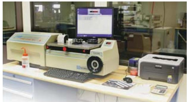
The ULM system maintains ultra-high accuracy by fully integrating a laser interferometer, zero Abbe offset design, and a large measuring table with center position, height, pitch, and yaw controls.
